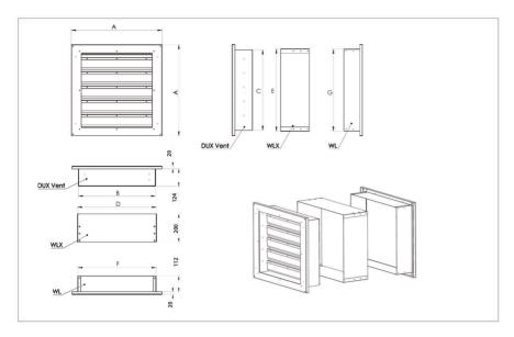
Standard kit fits walls from 100mm to 380mm thick.
