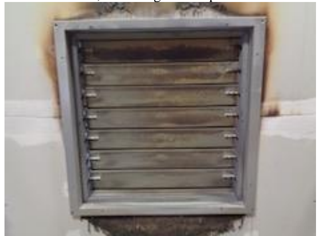
Post test: Unexposed side of test sample
