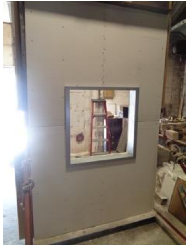
Wall construction, unexposed side
