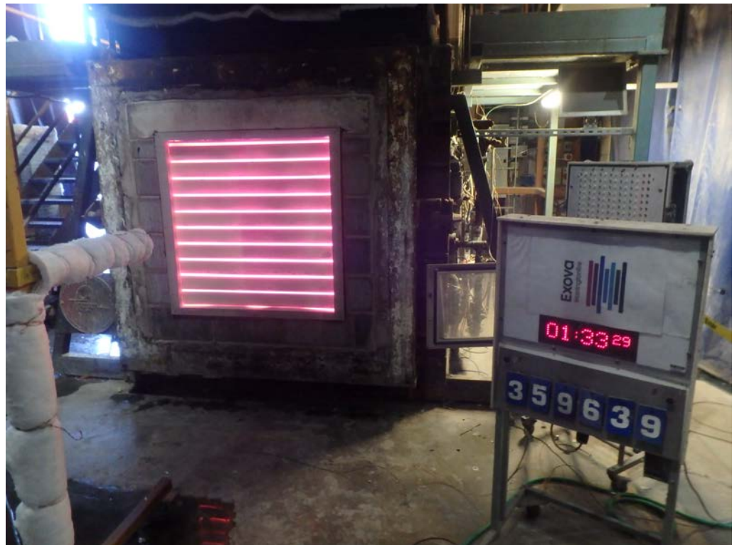
The unexposed face of the specimen after 93 minutes of testing
