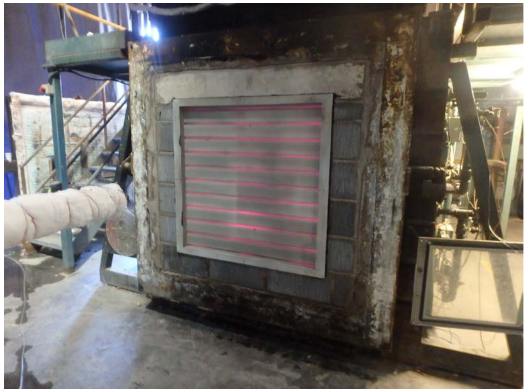
The unexposed face of the specimen after 30 minutes of testing
