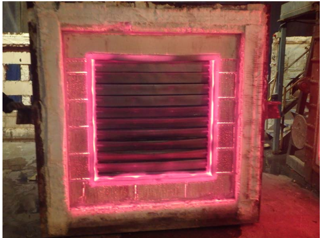
The exposed face of the specimen shortly after the test
