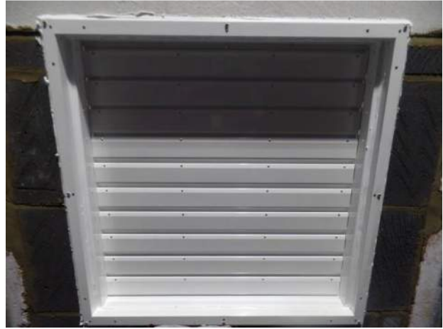
Exposed face of vent prior to testing
