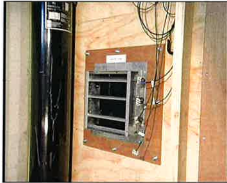
Photo of SHX 300 fully open in live gas discharge
