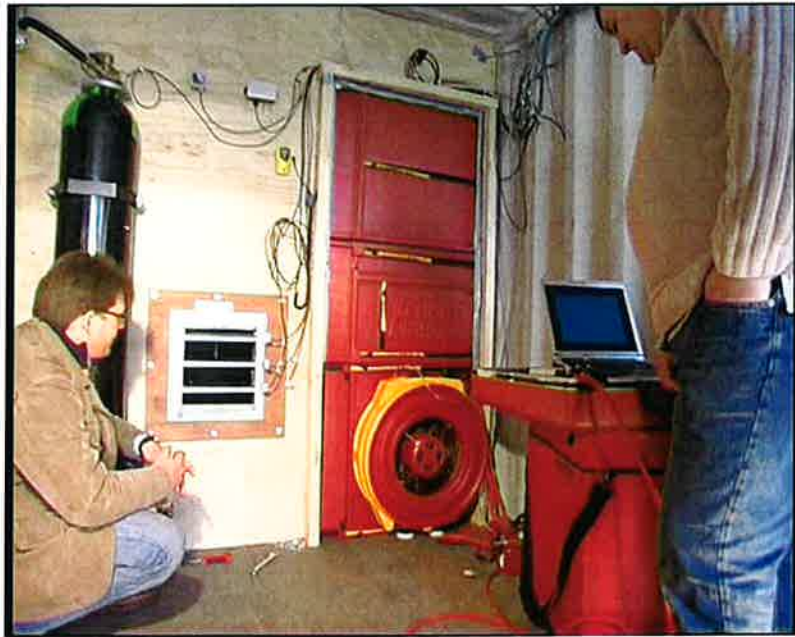
SHX Pressure Vent Being Tested
