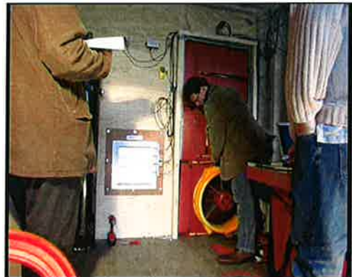
AES 300 fan test with holding kit in as pressure gets to 429 Pascal's
